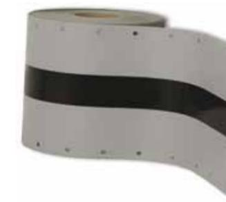
KÖSTER Joint Tape is a thermoplastic tape for waterproofing expansion joints. It comes in widths of 20 cm (for 12 cm wide joints) and 30 cm (for up to 20 cm wide joints). KÖSTER Joint Tapes are UV stable; highly elastic and can resist extreme joint movements.
