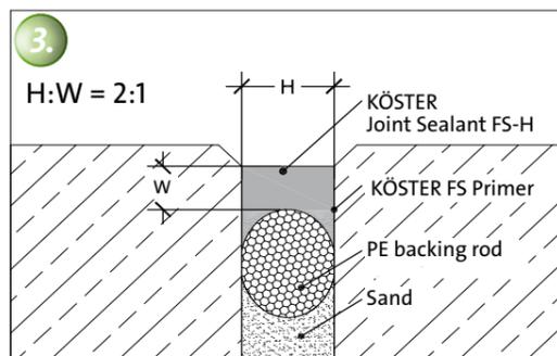
The Joint Sealant should be installed so that the ratio of joint height: width corresponds to the norm requirement. A detailed table is provided in the Technical Guideline.
