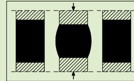
**Elastic** sealing compounds move back into their original shape after being stressed due to their extensibility. Sealing compounds for expansion joints should always be made from elastic materials. The more movement a joint experiences, the higher quality the waterproofing material needs to be.
