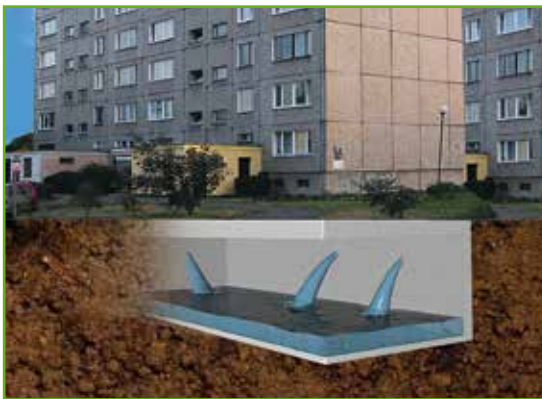
Basements often cannot be accessed from the outside. Thus they can only be waterproofed from the inside (negative side).
